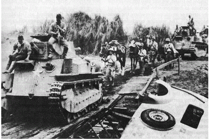
Type 89B medium tank of Col. Seinosuke Sonoda's 7th Tank Regiment is seen here crossing an improvised bridge erected to bypass Highway 6 north of Manila on 3 January 1942 during the fighting in the Philippines. This company used a white star as its unit insignia.
